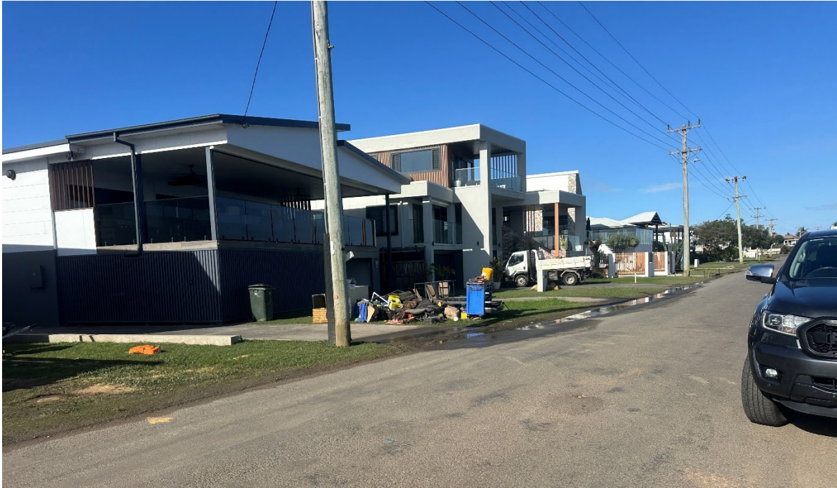
FIGURE 14 - ONE OF ONLY SEVERAL HOUSES ON SETTLEMENT POINT DRIVE, PORT MACQUARIE WITH FLOOD INSURANCE COSTING ABOUT $5000 PER YEAR. MOST HOUSES ON THE STREET ARE RAISED ON PIERS WITH LIVING AREAS LOCATED ON FIRST FLOOR AND GROUND FLOOR IS LARGELY A CONCRETE SHELL / GARAGE / STORAGE THAT ALLOWS WATERS TO PASS THROUGH
