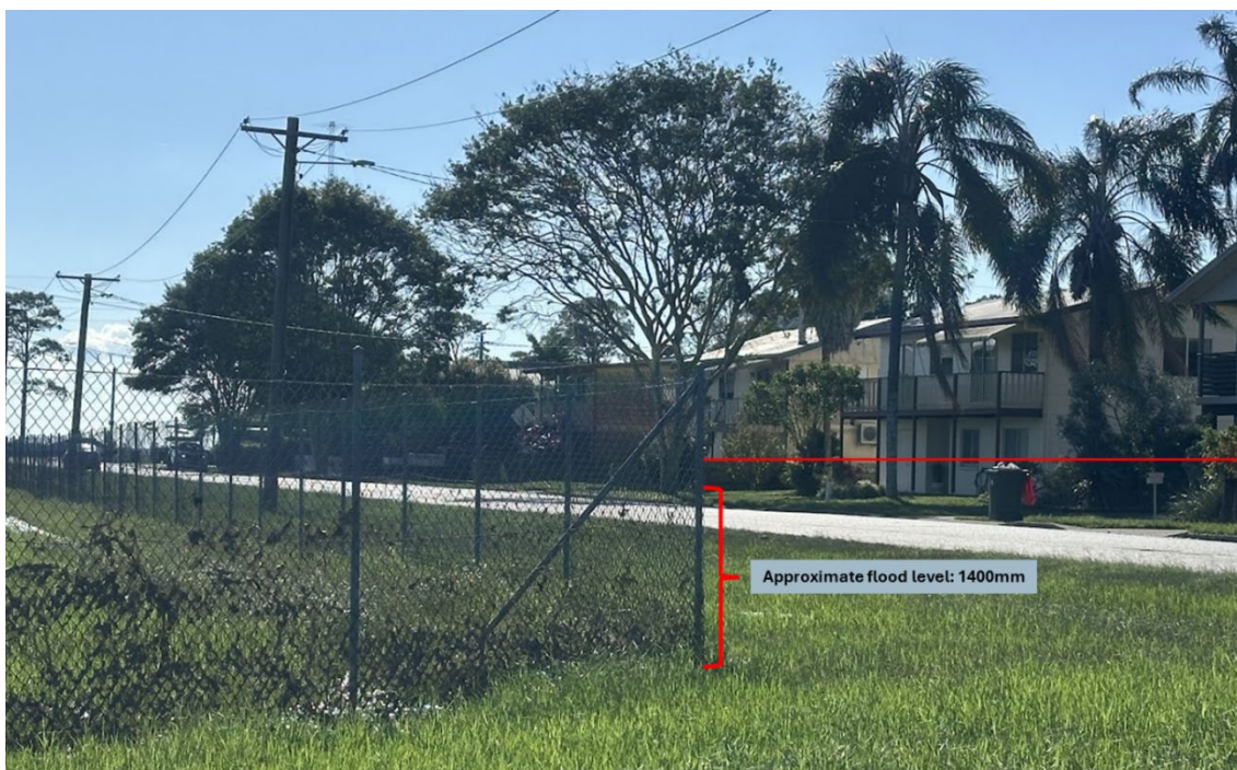
FIGURE 20 - RAWSON STREET AT SMITHTOWN SHOWING ABANDONED HOMES AND APPROXIMATE FLOOD HEIGHT OF 1400 MM (RED LINE) DETERMINED FROM FOOTBALL FIELD FENCE DEBRIS AND FLOOD WATER LINES ON HOMES
